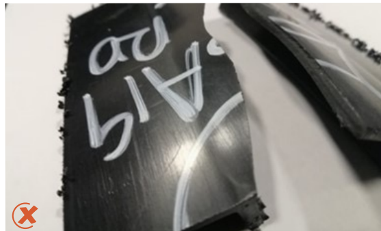
Injection moulded mudguard cracking in half
