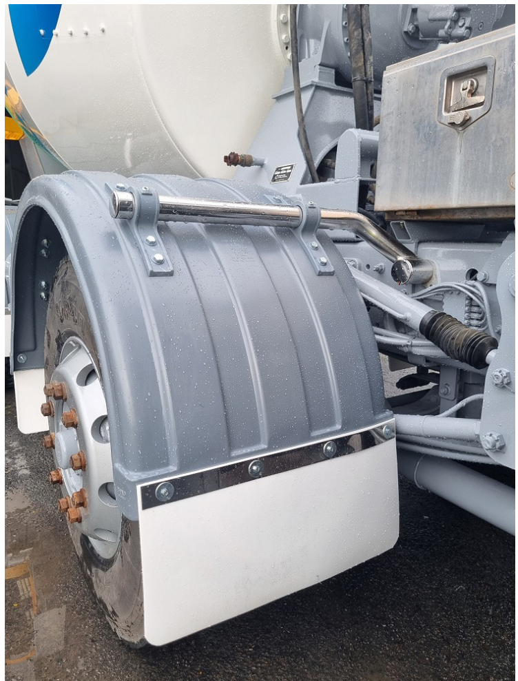
RHINO stainless steel chassis poles on concrete truck / agitator truck.
