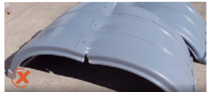
Injection moulded mudguard cracked
