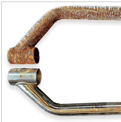
The RHINO salt spray test showing chassis poles – stainless (bottom) vs electroplated (top).
