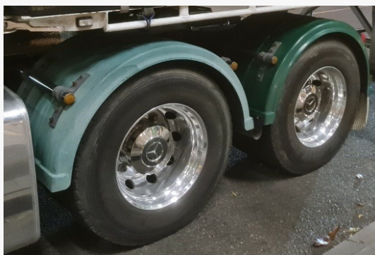
Popular competitor mudguard in Australia on a truck with one faded guard (left) and one new guard not yet faded (right). Notice the huge difference in colour between faded and unfaded.
