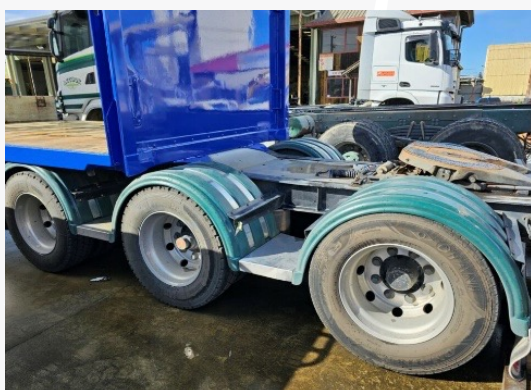
Trailer with RHINO Guards (9 years old); the colour has minimal fading.
